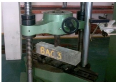
Fig.2. Bending Test on Beam
