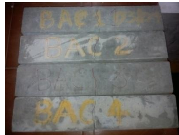
Fig.3 Crack Pattern in Beams
